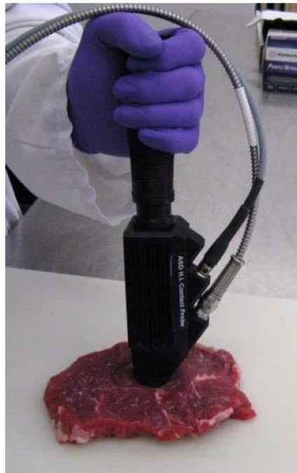
Figure 3. Collection of VIS-NIR spectra on intact beef samples using a portable LabSpec®4 spectrometer equipped with a fibre-optic high intensity contact probe.
